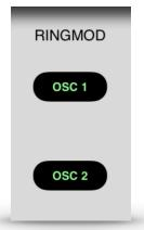
This module combines two input signals by multiplying them. The resulting spectrum contains the sum-of and the differences-between the frequency components of the two input signals. When the frequency of one input signal is below 20 Hz the result is a tremolo effect. But when the frequency is in the audible range the result is a change in timbre. If the pitch of the input signals are in an integer ratio to one another, the resulting spectrum is harmonic, otherwise the spectrum is inharmonic.
